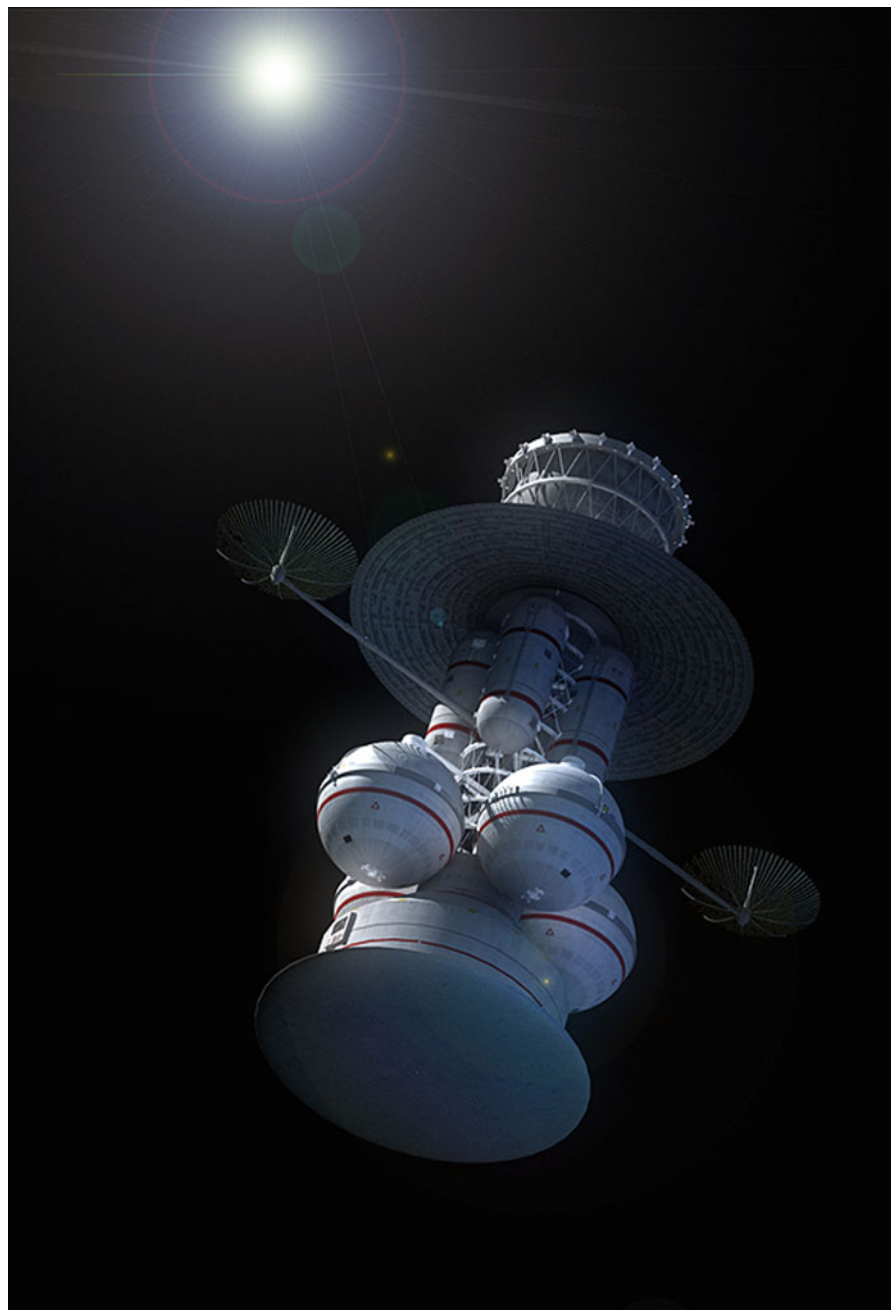
Plate 19 Project Icarus Starfinder probe. This artist illustration shows the Icarus Starfinder probe moving further from the Sun as it heads towards its 10,000 Astronomical Unit mission distance, deep inside the Oort Cloud. It is a proposal for a full technology demonstrator using a nuclear fusion based engine, paving the roadmap for an interstellar mission. Copyright: (@Adrian Mann/Project Icarus)
