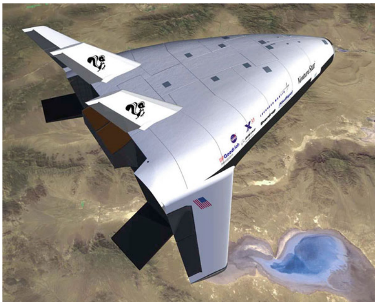
Plate 4 The US X-33 design. This was an unmanned sub-scale technology demonstrator for the VentureStar project, a planned next-generation reusable launch vehicle. It was developed by Lockheed Martin and included novel linear aerospike engines. It was cancelled in 2001. Copyright: (@NASA/courtesy of nasaimages.org)
